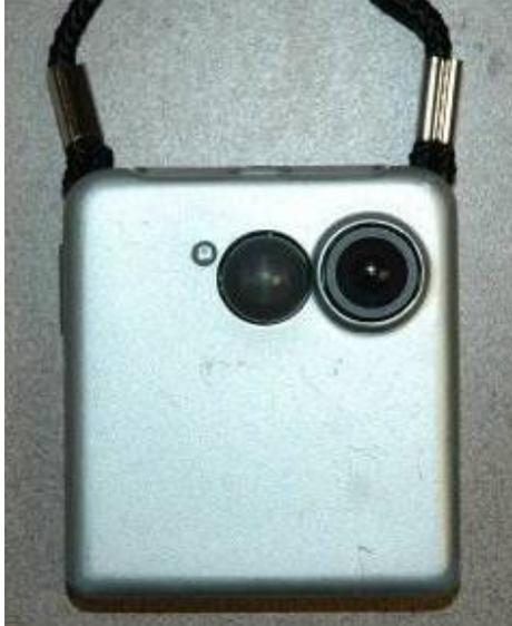
**Figure 1. SenseCam (64x71mm body)**
